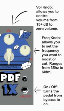
• Parametric EQ with adjustable volume can boost the clean channel of an amp into distortion and clipping with the option of additional clipping from the gain circuit.
